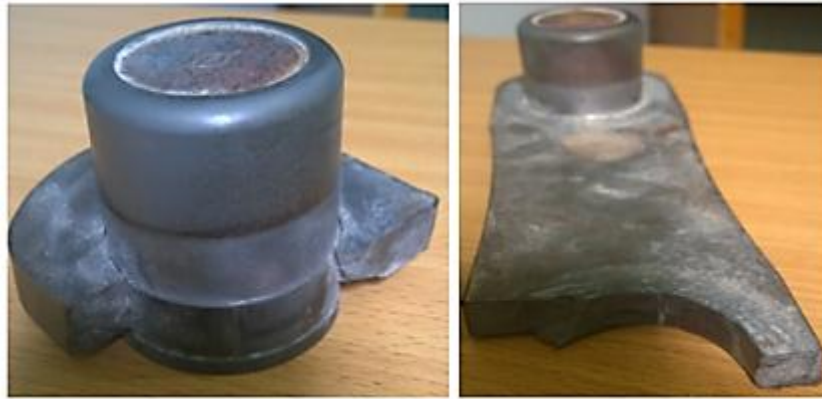
Figure 4: Failed chain links.
