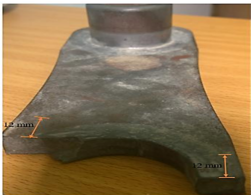
Figure 2: Sectioning of failed sample.
